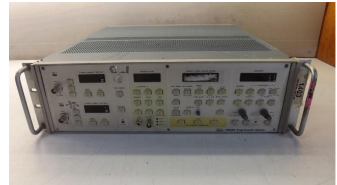
Sony Tektronix 390 AD from 1982 Still used in LI measurements Newer digitizers are only somewhat better
