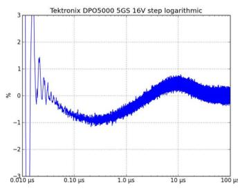
For a full lightning impulse, the step needs to be within 1% from 0.42  $\mu\text{s}$  to 60  $\mu\text{s}$ . This time scale is difficult to observe when using linear plots, as the 0.42  $\mu\text{s}$  point will be difficult to discern. When using a logarithmic scale, the 0.42  $\mu\text{s}$  point is easy to identify. The exact 60  $\mu\text{s}$  point is harder ascertain, however this is of little consequence since the step response in general has stabilized at that time.
