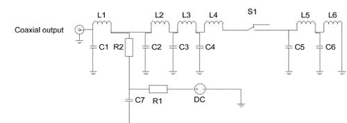
A detailed equivalent circuit of the switching circuit of the step generator is given in figure above, where inductance in the leads and capacitance to earth are shown as a ladder type network. The values are possible to estimate only to order of magnitude, and serve as a help in understanding. L1 to L6 as well as C1 to C6 are estimated from geometrical dimensions.
