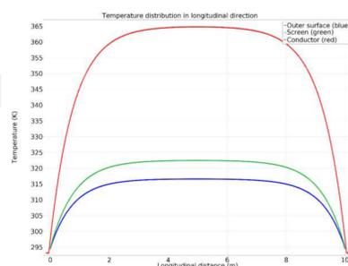
Fig. 3. The temperature distribution along the cable conductor (red), screen (green) and outer surface (blue) in the ac circuit.
