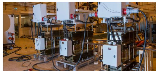
Fig. 6. SP's new ac current generators can supply up to 10 kA and 15 V compliance each.
