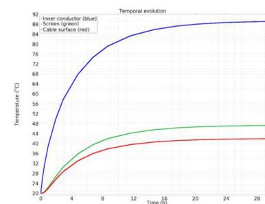
Fig. 4. The temperature of the conductor (red), screen (green) and outer surface (blue) of the cable in dc circuit during warm up.
