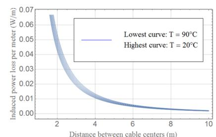
Fig. 5. The power loss in the dc circuit due to the induced ac current can be neglected compared to the self heating, which is approximately 90 W/m, if the distance between the cables are >2 m.
