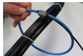
Magnetic ring around the probe junction
