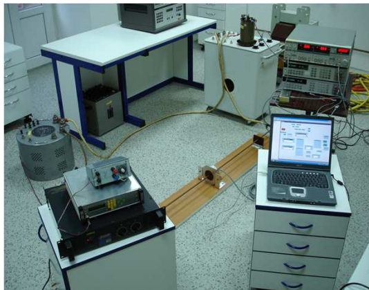
Fig. 2. Working place for Rogowski coil calibration
