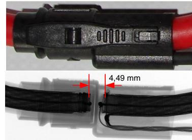
Fig. 2: Lock of a Rogowski coil (photo and X-ray photo) [2]
