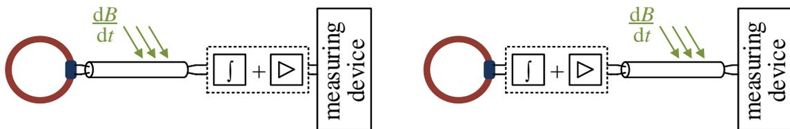
**Fig. 6:** Setup with signal integration and conditioning close to the measuring device. **Fig. 7:** Setup with signal integration and conditioning close to the Rogowski coil.
