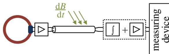
**Fig. 8:** Setup with using a preamplifier close to the Rogowski coil.
