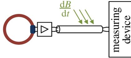
**Fig. 10:** Setup without using an analogue integrator.
