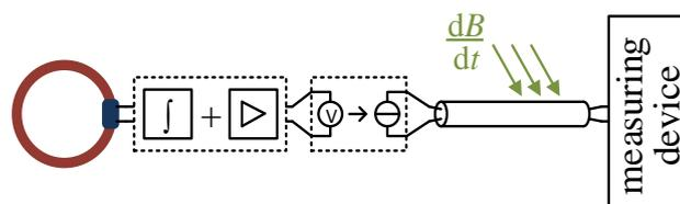
**Fig. 9:** Setup with using a voltage to current transducer.
