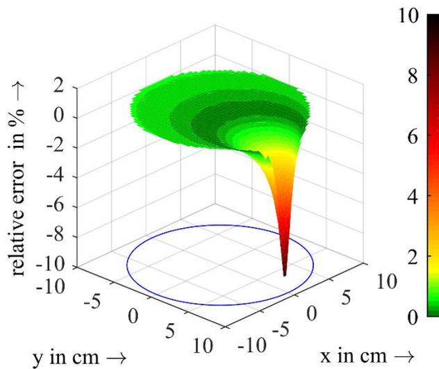
Fig. 3: Relative error dependent on the position of the primary conductor [2].
